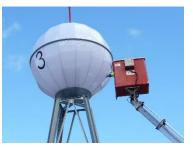
Positioned at the top of the mast, at a height of 8m, a **LumiSphere** containing 4 lamps 1000W provides an illumination level of 11 lux at 55m (circular area of 10000 m<sup>2</sup>)
